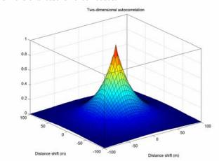
Figure 2: Autocorrelation of shadowing as a function of distance shift (movement in two dimensions).
