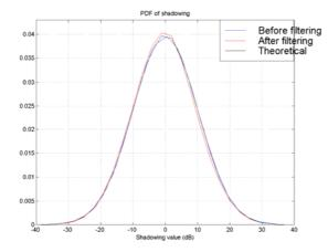
Figure 4: Probability density function of simulated shadowing.
