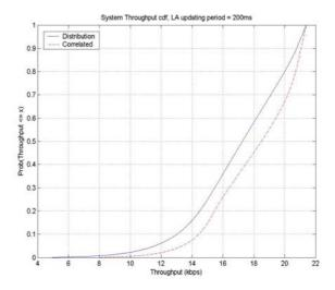
Figure 7 – System throughput cdf for a LA updating period of 10 RLC blocks (200 ms).
