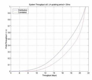
Figure 6 – System throughput cdf for a LA updating period of 1 RLC block (20 ms).
